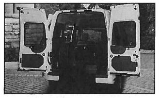
With the rear tumble seat folded forward, the vehicle's design provides a wheelchair area of 31" wide x 50" in length. With the rear seat in its deployed position, three full-sized adults can be transported in the rear seating area, along with the driver and another passenger in the front. This new design combines the flexibility of a rear entry transport van for handicap passengers with non-wheelchair passenger capabilities, transitioning from one use to the other in less than a minute.
